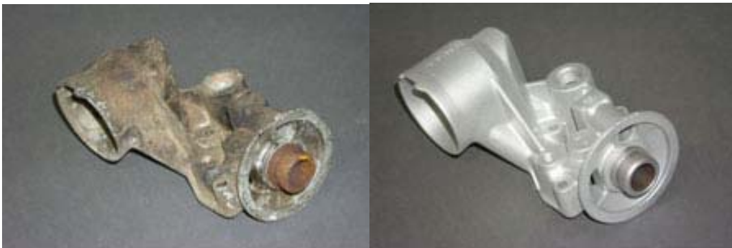
Figure 1: Cast component before and after cleaning
