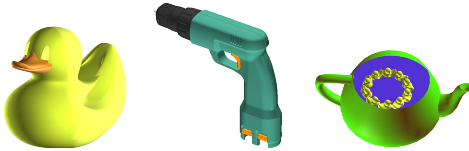
Fig. 1. NURBS models constructed from trimmed NURBS surfaces evaluated and rendered on the GPU.
