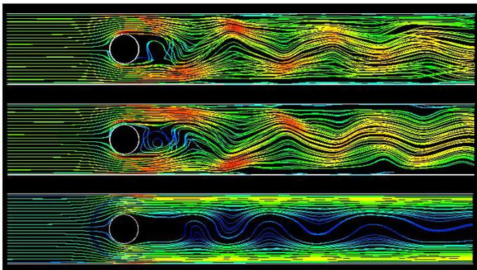
Figure 9 : Path Lines colored by X-Velocity for 5mm, 3mm and 1mm Fin Spacing
