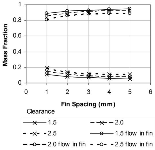
Figure 8 : Flow rate fraction through fins
