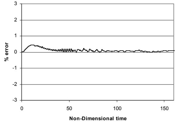
**Figure 6 : Difference in average heat flux for 2mm fin space between two grid sizes**
