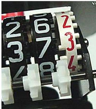
**Figure 3 Helper wheel engage with pegs**
