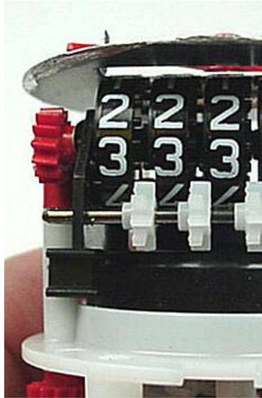
**Figure 2 The helper gears on the auxiliary shaft**
