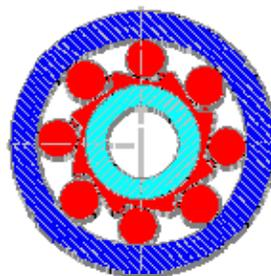
**Figure 6 Roller Ramp Freewheel**
